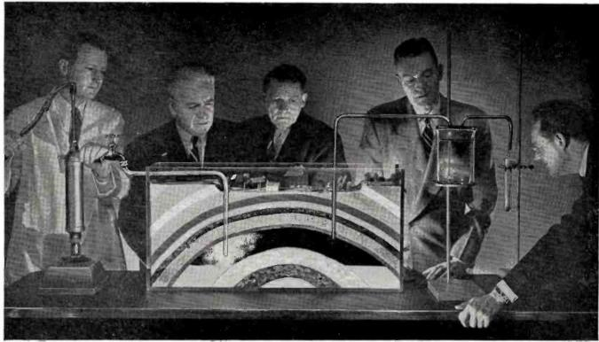
OIL SCIENTIST, using laboratory model, shows how water flooding revives oil fields which have lost natural "push." By pumping water into oil-bearing sands, trapped oil is forced toward outlet wells which bring it to the surface,
